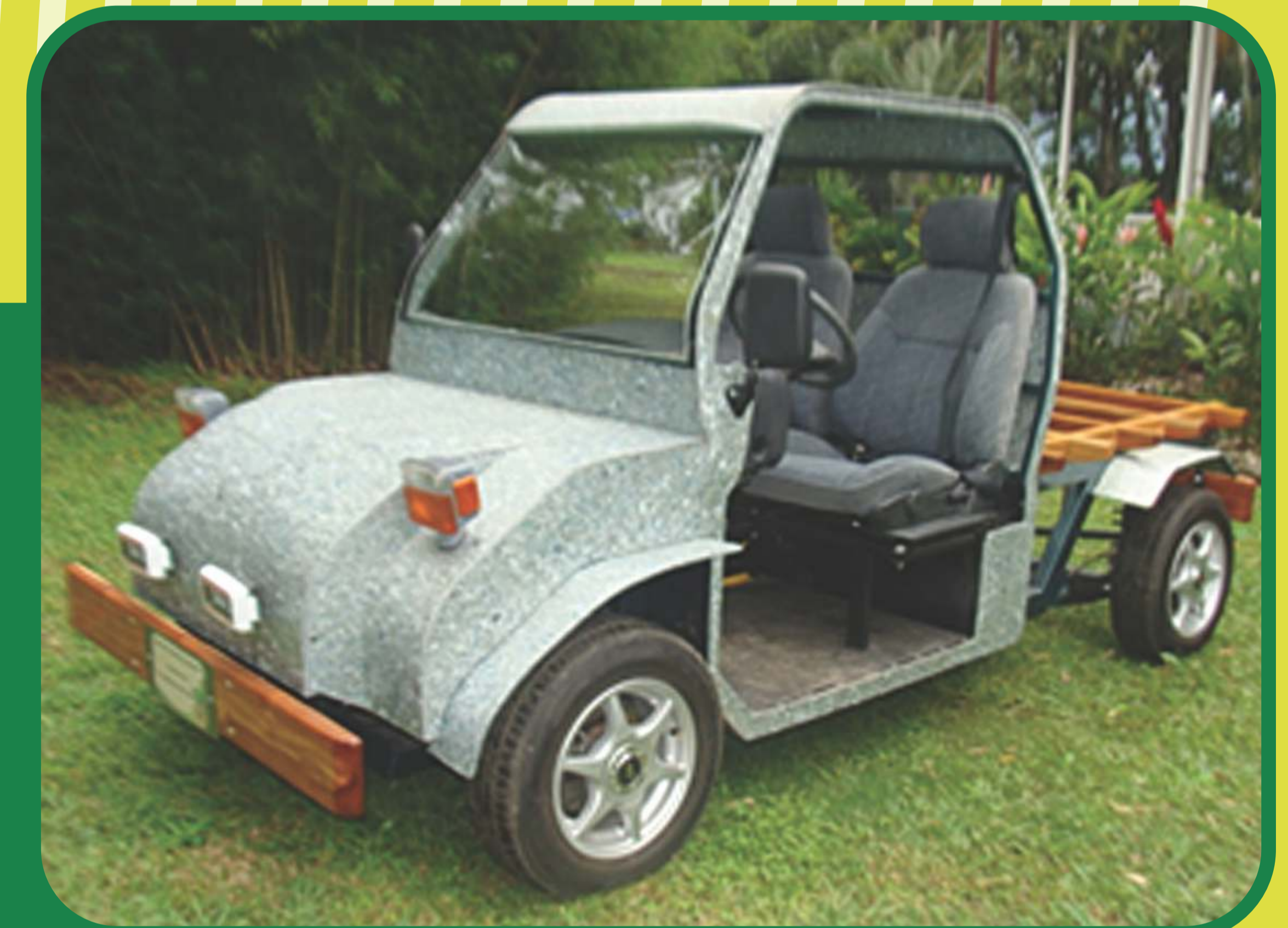
An electric vehicle prototype built at the Costa Rican National Training Institute with parts from other vehicles, the original design of the chassis, and the bodywork is constructed from tetra pack and other packaging waste collected from a dairy cooperative
