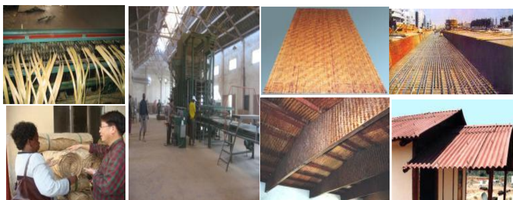
Fig. 59. Bamboo boards for concrete boards and corrugated roofing
