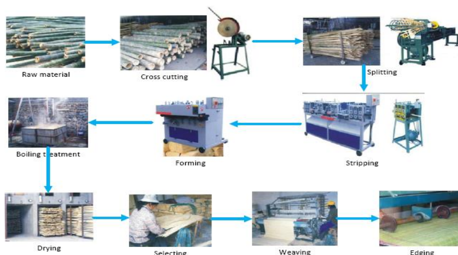
Fig. 38. Processing technology flow of bamboo curtain, mat and carpet
